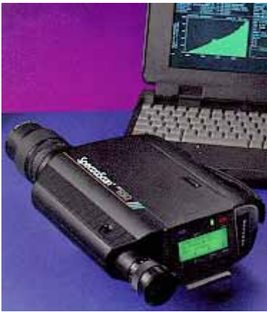
Figure 9 : PR650 instrument PR®-650/640 SpectraColorimeter™ System.
