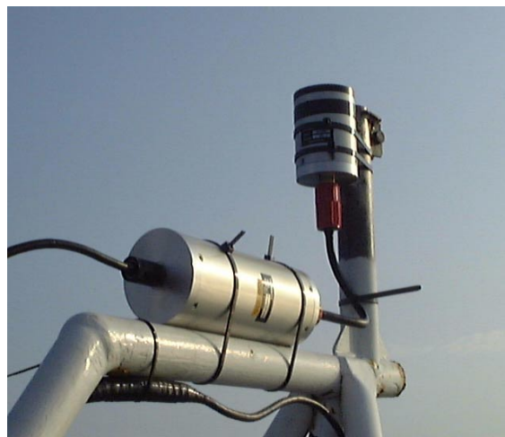
Figure 6: Satlantic sensor head for E_s(\lambda) measurements.
