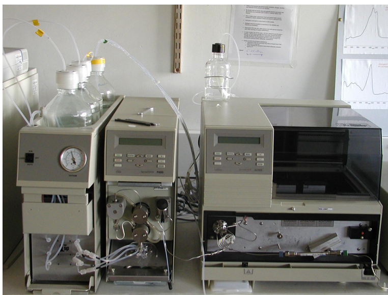
Figure 5: Diode array detector (UV6000LP) and pumping system (P4000) for High performance liquid chromatography.
