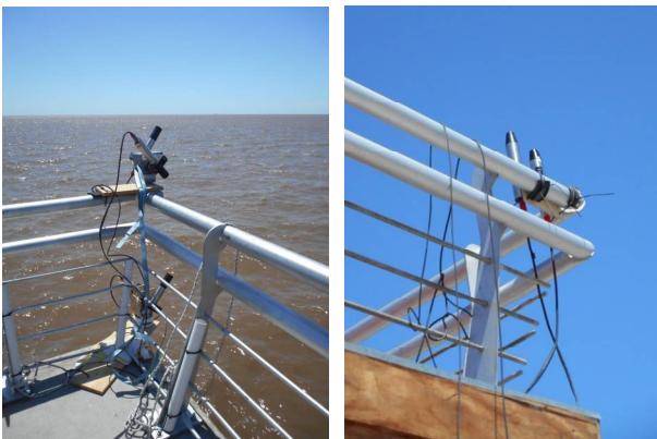
Figure 3. Setup of the two Trios/RAMSES sensors at the end of the Fishermen Pier (Argentina). Radiance (left) and irradiance sensors (right).
