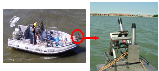
Fig. 5: TriOS optical sensors mounted on the Rigid Inflatable Boat, called the Tuimelaar.
