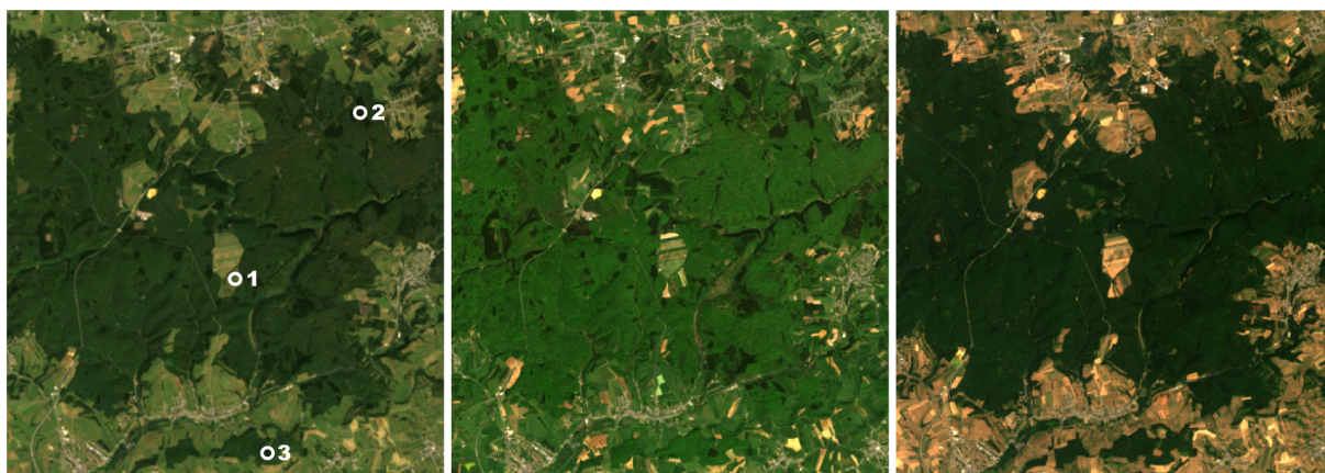
Fig. 2. L8/OLI \rho_s RGB composites for the BUZENOL ROI (site 13), cloud-free mission median (left) and images for 2014–05-05 (middle) and 2018–08-04 (right). All three images have the \rho_s R (655 nm), G (561 nm) and B (483 nm) linearly scaled from 0–0.15 to the 8 bit RGB channels. Scene dimensions are approximately 12 by 12 km. The left plot shows the locations of the emissivity time-series in Fig. 8, (1) Field, (2) Pine, (3) Pine cut in 2018.
