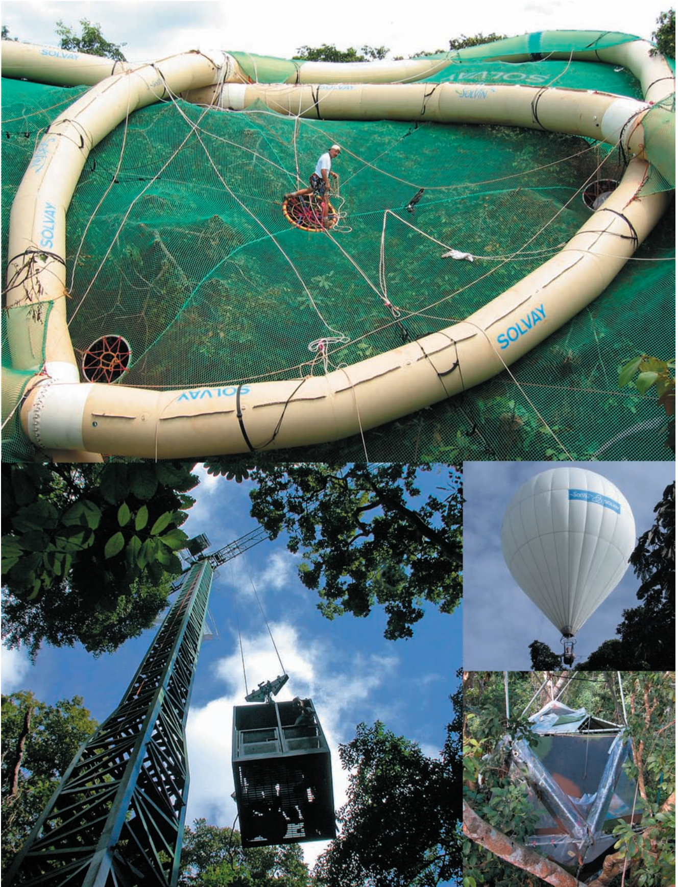
Plate 2 — Canopy access devices, clockwise: SolVin-Bretzel canopy raft, canopy bubble, Ikos tree house and canopy crane. Photos: S. Bechet, R. Le Guen, JO, ML.
